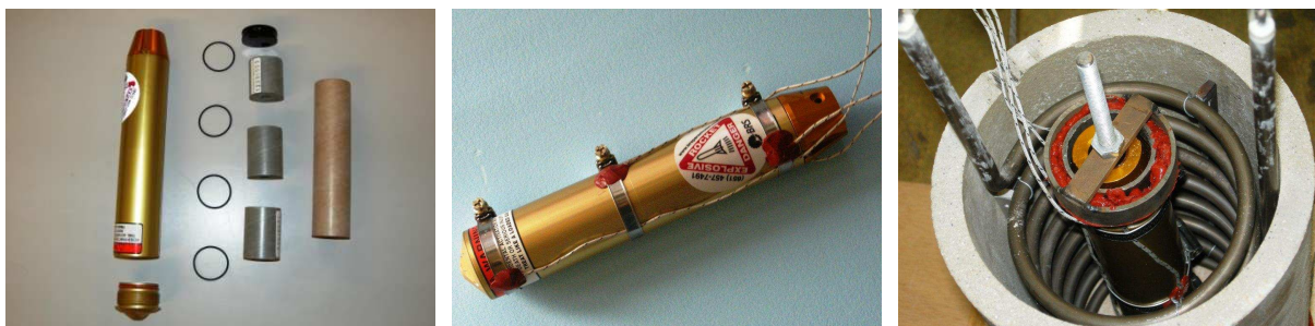
Fig. 8: Arrangement of the BRS 440 rocket for the SCO test; respectively rocket with probes and in position in the brick cylinder.
