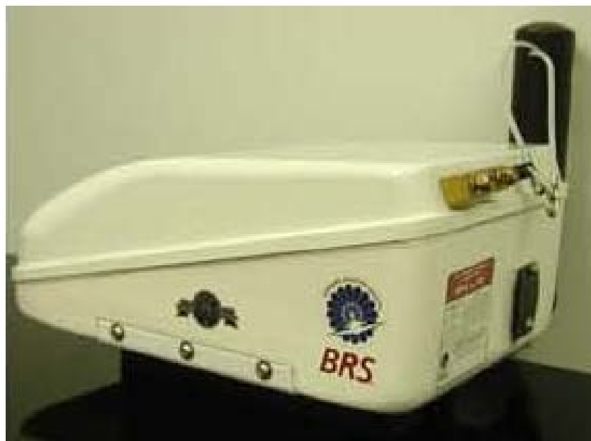
Fig. 7: Parachute packed in rectangular container (VLS)
