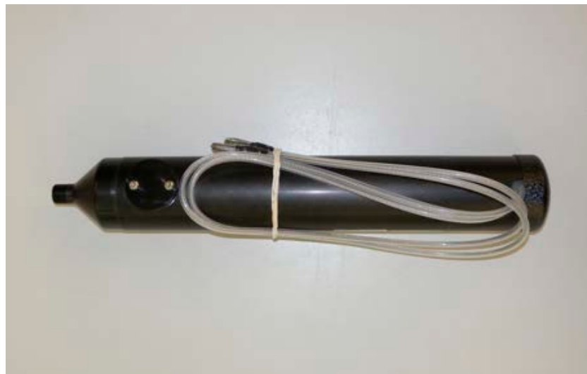
Fig. 11: Rocket motor with release/igniter unit
