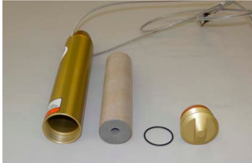
Fig. 10: Stripped down rocket motor
