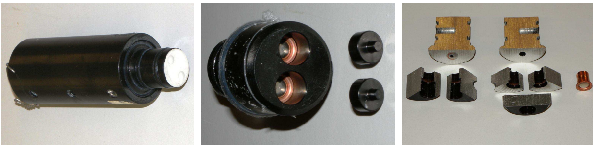
Fig. 2: Detail of the igniter of the BRS 440 rocket. The primary booster charge is contained in two firing channels under an aluminum foil (glued to the base of the igniter; left picture). The picture in the middle shows the two percussion cups in the igniter housing and the two firing pins beside. The rightmost picture shows one of the two percussion cups and the housing cut by a diamond wire saw.
