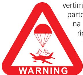
This aircraft is equipped with a ballistically-deployed emergency parachute system
