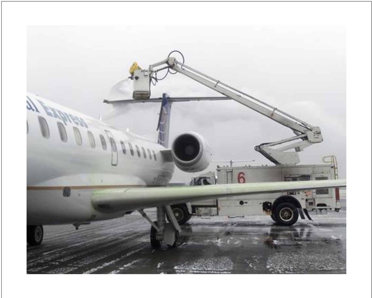
Figure III-10-1. Typical de-icing/anti-icing ground equipment (Image reproduced by kind permission of NASA.)
