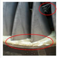
Parts of temporary repair ingested into engine.
