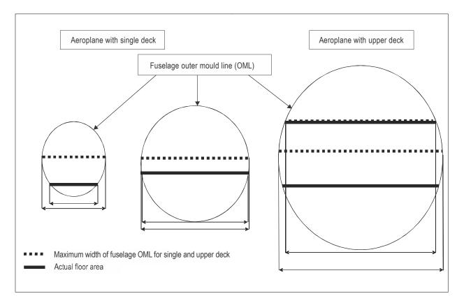
Figure A2-1. Cross-sectional view
