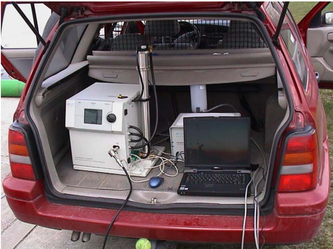
Picture 5: SMPS (on the left) with DMA (the vertical tube). The CPC is installed behind the Laptop.
