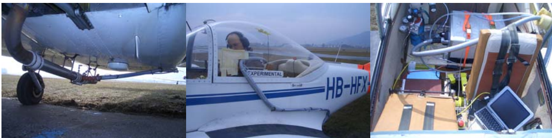
Exhaust flow meter, heated sampling line and installation on backseat of HB-HFX
