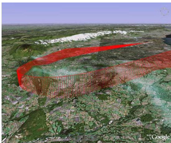
Picture 3: Approach path of a selected flight for ADAECAM validation in a three dimensional view. The LTO approach segment below 3000ft AGL is the last straight path down to the runway. [Picture from Google Earth™, not to be used for commercial purposes]
