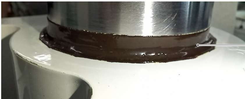
Nose Landing Gear - Cylinder Pipe - Repair Figure 4
