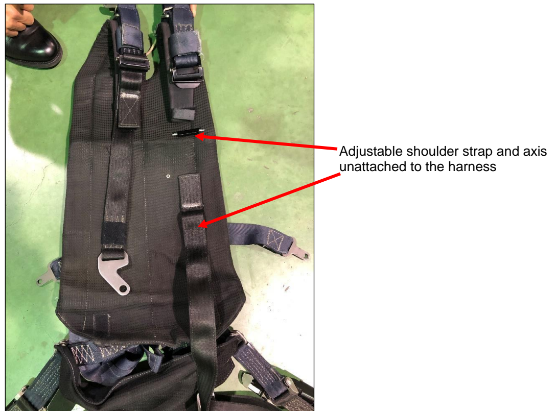
Figure 2 – Customer notification (shoulder straps and axis unattached)
