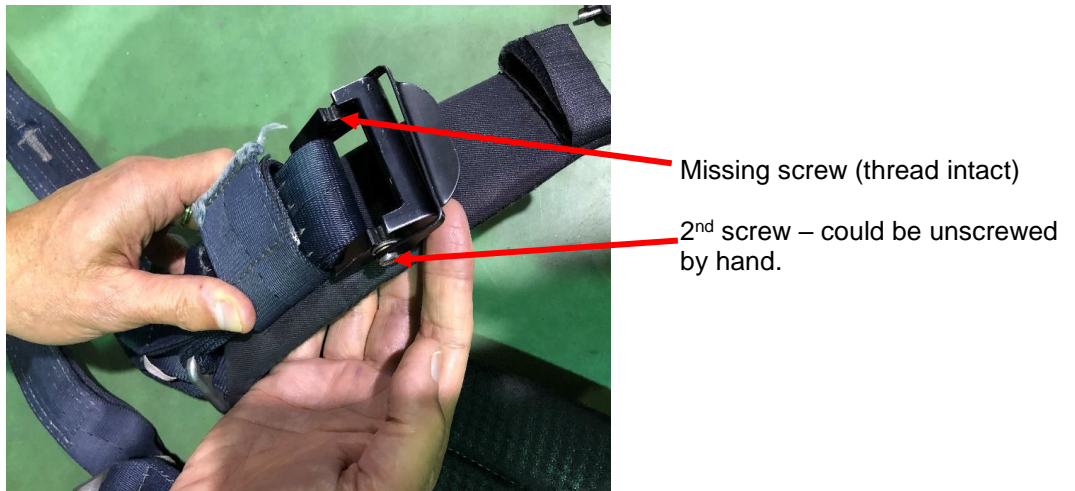
Figure 1 – Customer notification (missing and loose screws)
