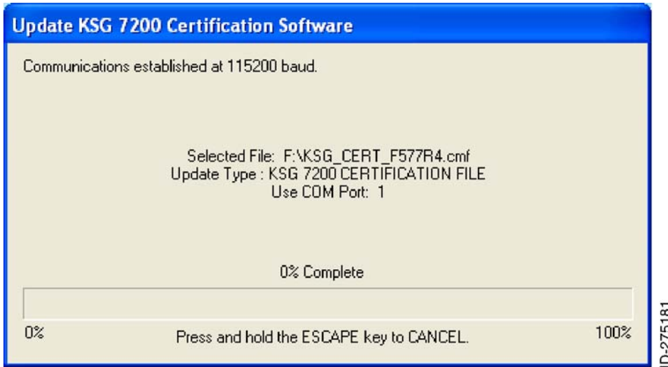
Figure 36. (Sheet 1 of 1) Update KSG 7200 Certification Software Window for Pilatus Certification File KSG_CERT_F577R4.cmf (60/75 mGauss settings)
