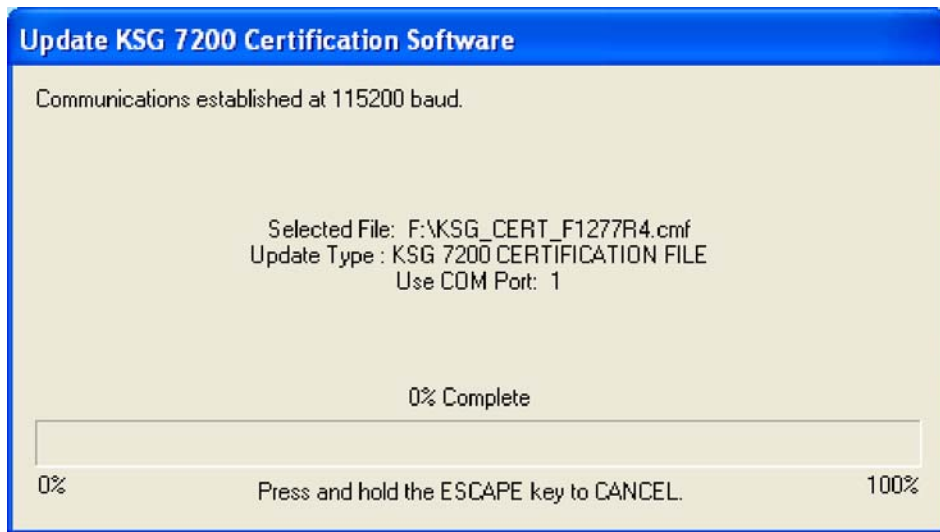
Figure 39. (Sheet 1 of 1) Update KSG 7200 Certification Software Window for Twin Otter Certification File KSG_CERT_F1277R4.cmf (Certification File 3a)
