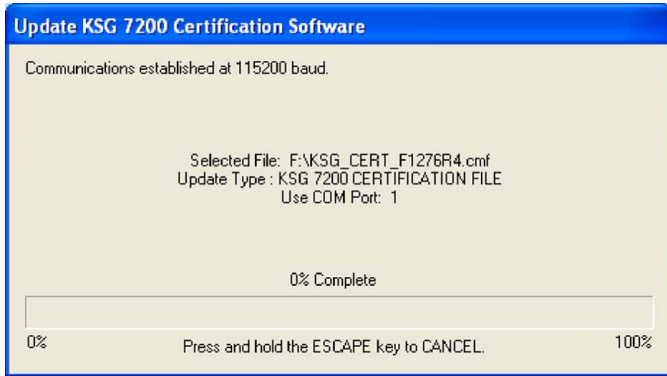
Figure 38. (Sheet 1 of 1) Update KSG 7200 Certification Software Window for Twin Otter Certification File KSG_CERT_F1276R4.cmf (Certification File 2a)
