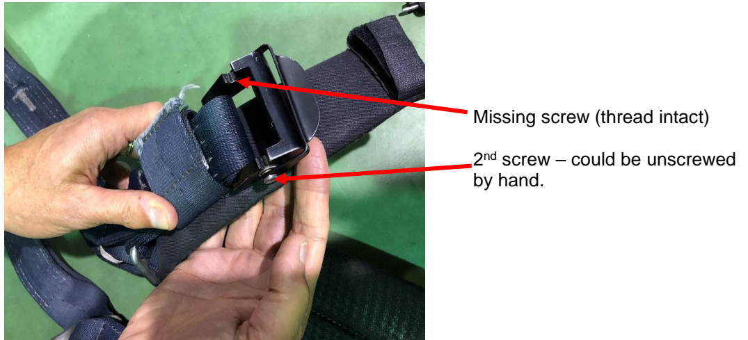
Figure 1 – Customer notification (missing and loose screws)
