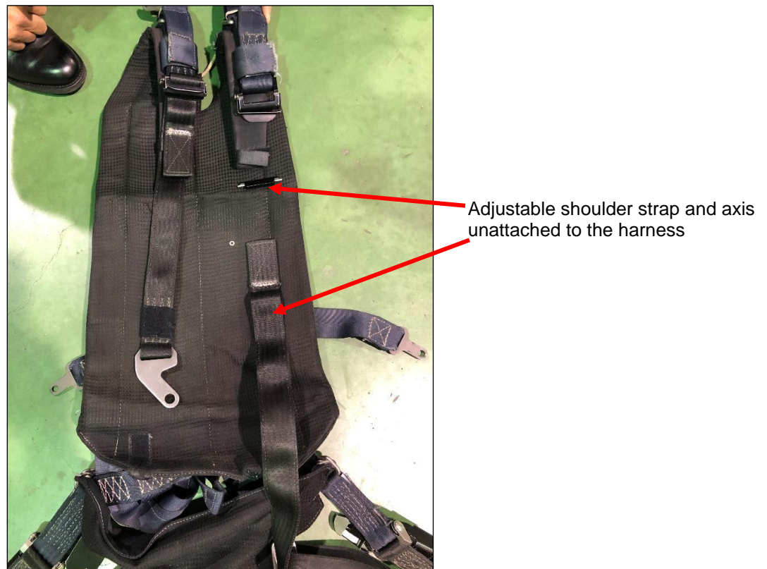
Figure 2 – Customer notification (shoulder straps and axis unattached)
