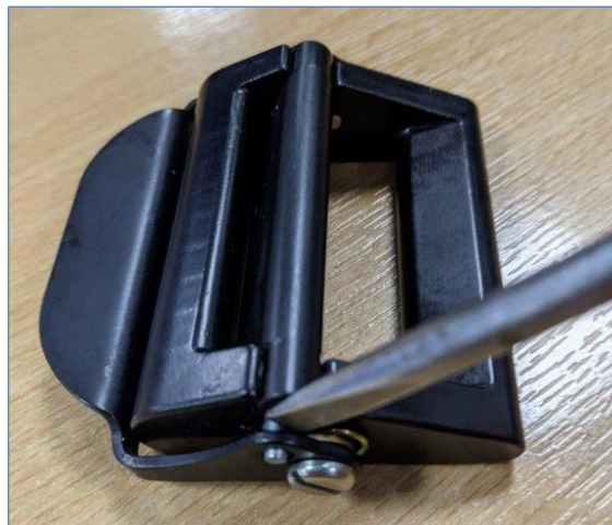
Fig 3 – Use of small flat blade screwdriver to hold spring in place
