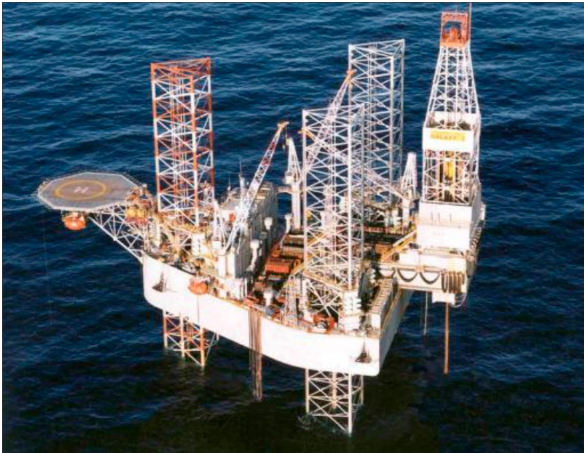
Figure I-1-3. A three-legged jacked-up mobile offshore drilling unit
