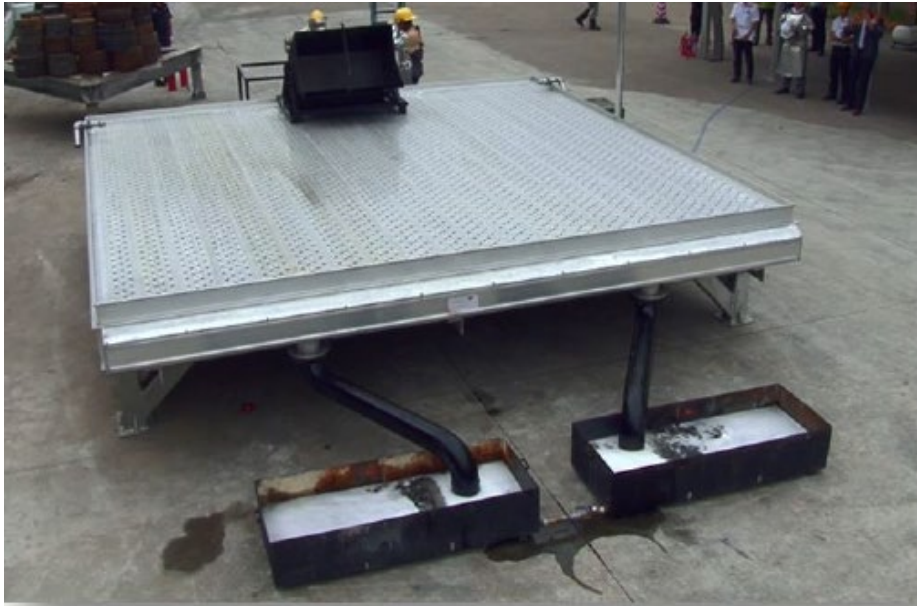
Figure II-6-7. A fire test on a passive fire-retarding surface (180 L of fuel is collected)
