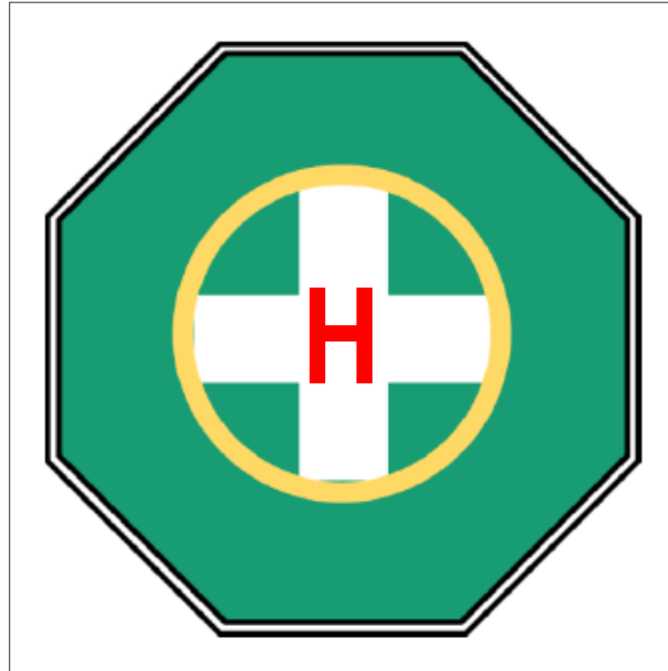
Figure II-5-4. Heliport identification marking with TDPC (hospital)
