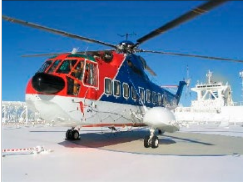
Figure I-5-1. S61N operating to a non-purpose-built ship's side heliport
