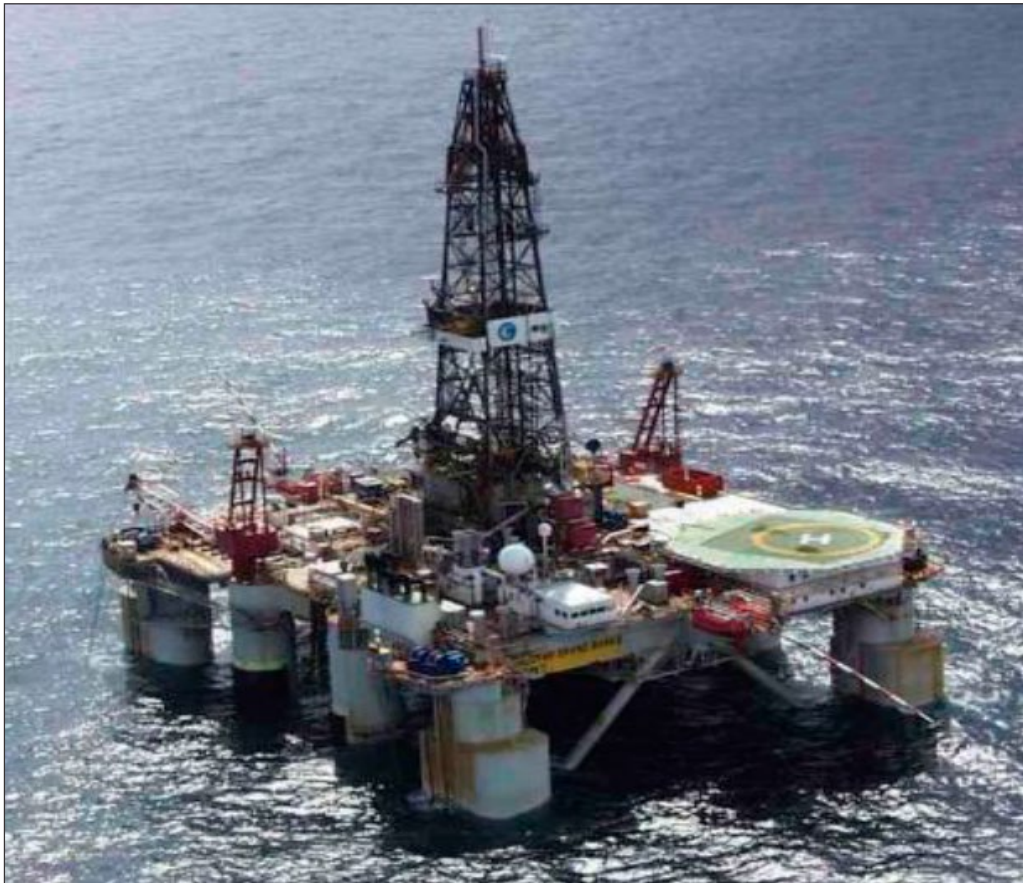
Figure I-1-2. A deep ballasted semi-submersible mobile offshore drilling unit
