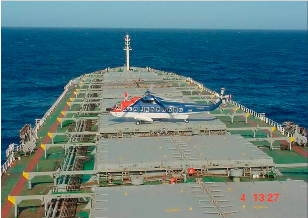
Figure I-1-9. An S61N helicopter lands on the hatch cover of a large vessel
