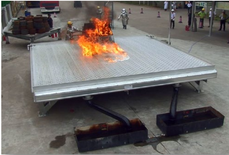
Figure II-6-6. A fire test on a passive fire-retarding surface (200 L of burning fuel)
