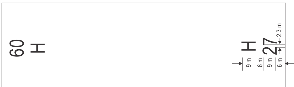
Figure II-5-11. Designation markings for runway-type FATO
