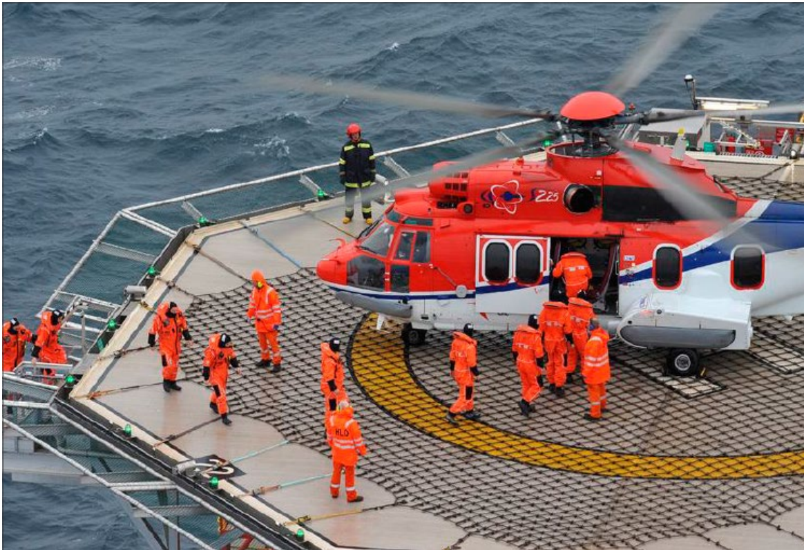
Figure I-5-6. Accurate positioning of a helicopter by correct use of the touchdown/positioning marking (TD/PM) circle
