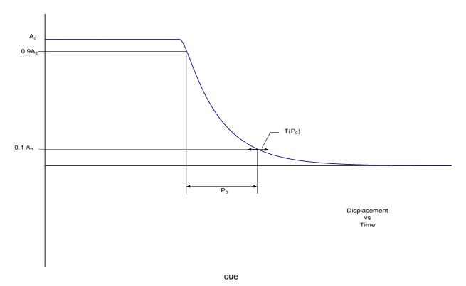
Figure 2: Critically damped step response
