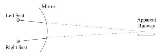
Figure 2 - Runway view in a collimated display
