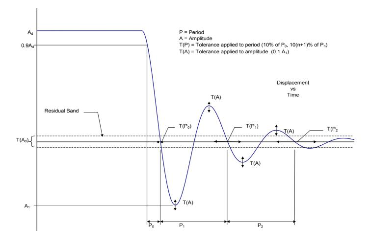
Figure 1: Underdamped step response INTENTIONALLY LEFT BLANK
