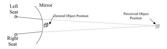
Figure 4 - Near field object in a collimated display
