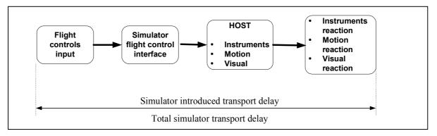
Figure 1: Transport Delay for simulation of classic non-computer controlled aircraft
